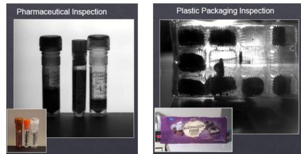
**Figure 9.** (Left) Image of vials with a clear water-based liquid with the liquid appearing dark due to the SWIR absorption feature around 1420 nm. The inset shows the same vials with a visible camera. (Right) Inspection images of a food product where the SWIR photons are used for their increased transmission through plastics and dyes. Inset shows the product imaged with a visible camera.
