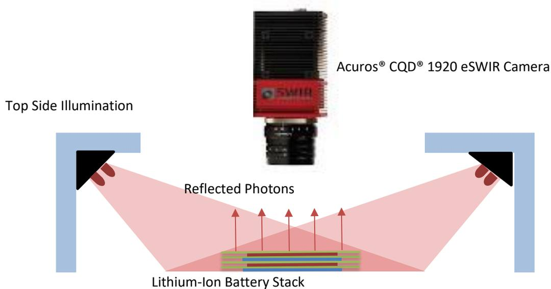
Figure 2. Typical battery inspection setup showing a "stacked" type cell with alternating Anode/Cathode (blue & red) layers with polymer separator (green) between each interface. Incident SWIR radiation illuminates the sample and the light reflected back to the SWIR image sensor provides detail regarding the subsurface layers covered by the separator.
