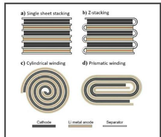
**Figure 1. Schematic showing four typical types of Li metal batteries manufacturing processes. (a) Single sheet stacking; (b) Z-stacking; (c) cylindrical winding and (d) prismatic winding.**
