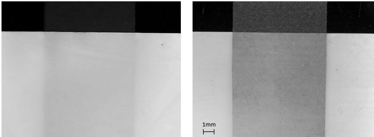
**Figure 3. Visible (left) and SWIR (right) images of lithium-ion anode layer as viewed through a polymer separator. Because the polymer separator material is more transmissive in the SWIR spectrum, the anode edge is clearly visible in the SWIR image on the right versus the faint shadow detected by visible image on the left.**
