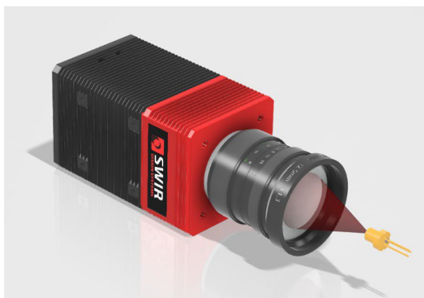
Figure 1. CAD Depiction of a Near Field Imaging Setup Showing a SWIR VISION SYSTEMS Camera Equipped with a Lens and Focused on the Emitting Aperture of a Lasing Laser Diode
