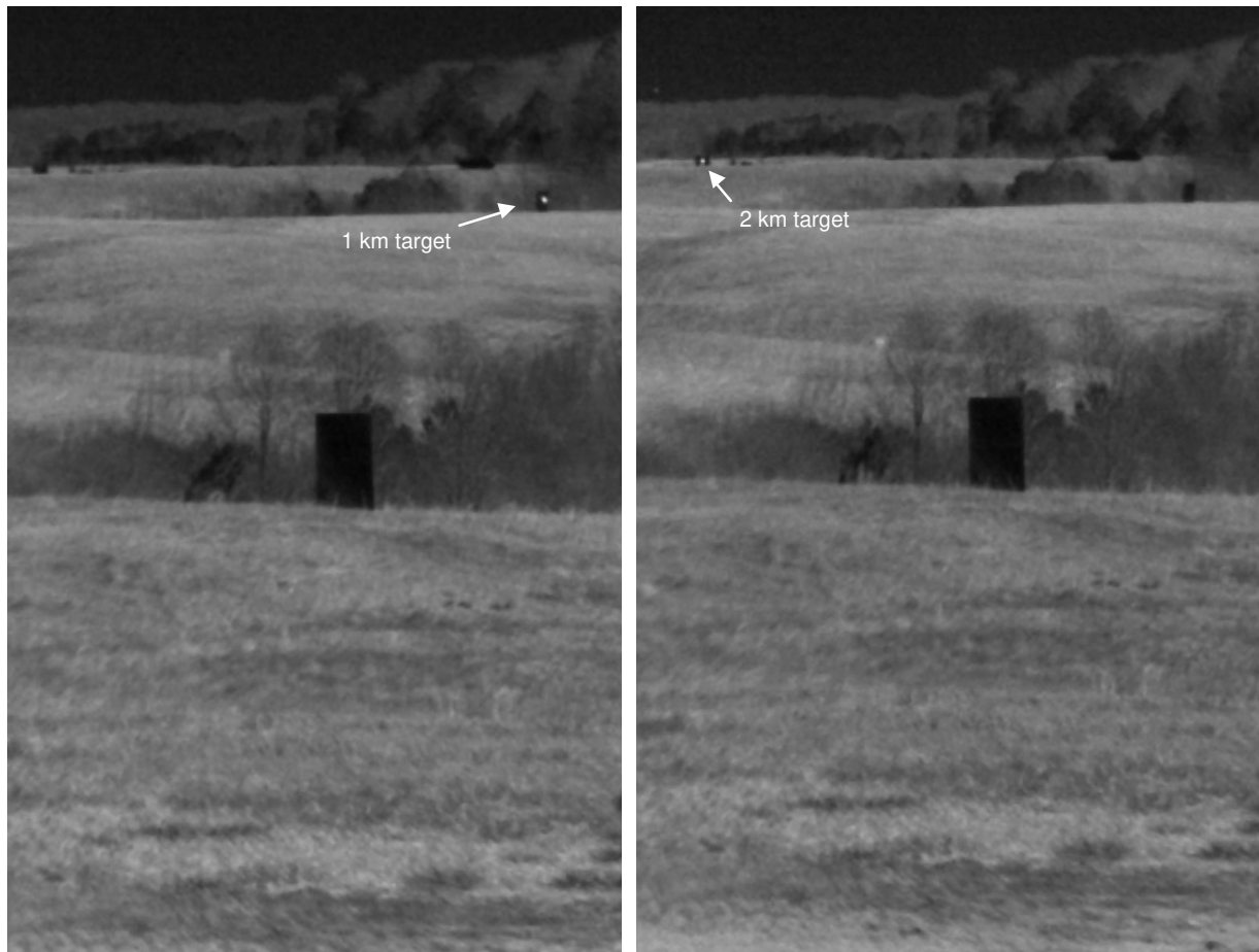
Figure 7. 1550 nm Laser Ranging in Full Sunlight at 1 km and 2 km Target Distances Using an ACUROS SWIR Camera
