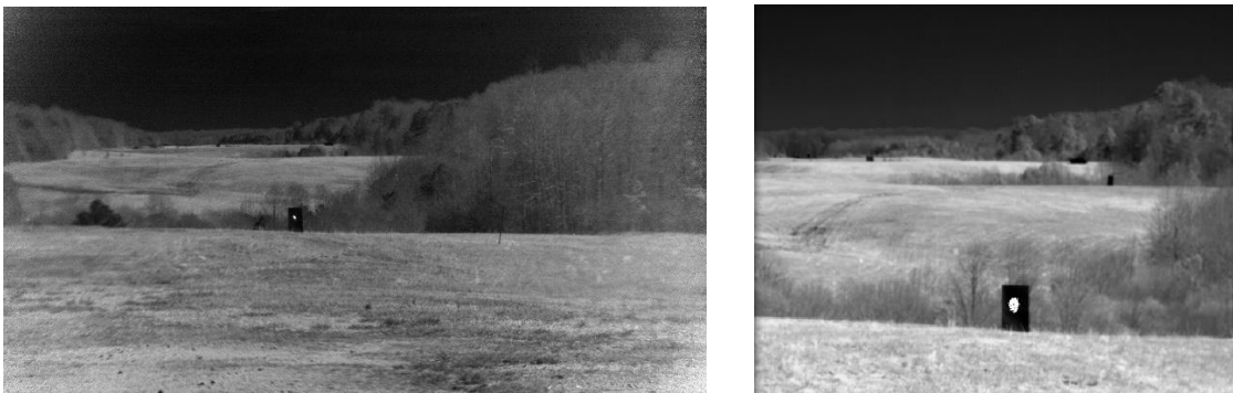
Figure 12. Comparison of CQD (Left) and InGaAs (Right) Cameras Imaging 200 m Target
