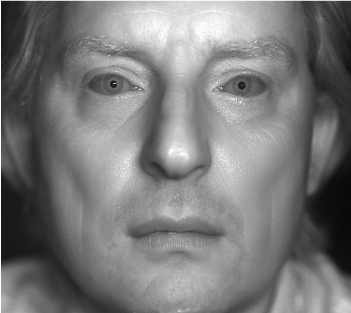
1150 nm LED, 5 ms exposure
