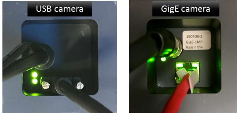
Figure 9. Acuros CQD Camera back panel after communication and power have been supplied.
