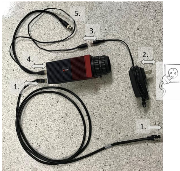
Figure 8. Acuros CQD Camera cable connections. Connections should be made in the listed order.
